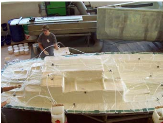
The deck is produced using the vacuum infusion method
