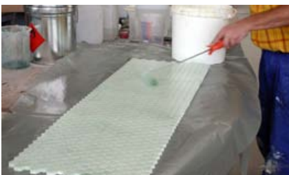
Hand lay-up laminate
