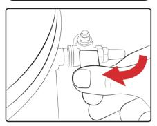
Make sure the inlet valve (which has the brass filter fitted) is in the closed position. especially if you have just run a degassing operation.
