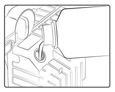
Unlike conventional oil-bath vacuum pumps, the *EC20* emits virtually no oil from the pump during operation however, depending on how frequently you use your vacuum pump and how you are using it, you still need to periodically check and top-up the oil level to ensure it stays at the recommended level.
