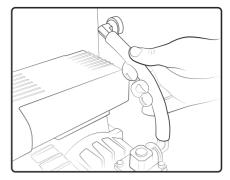
Connect the vacuum pump to the chamber by pushing the hose firmly onto both hosetail fittings.
