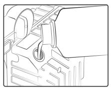
The *EC20* pump ships without oil and needs to be filled to the correct level using the supplied oil before use.
