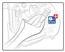
Tightly screw the 90° brass elbow fitting into the 1/2" port on the *EC20* vacuum pump. Finish with the fitting facing upwards.
