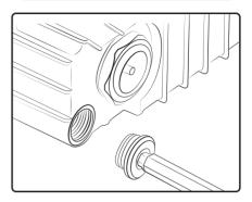
If the oil appears cloudy, discoloured or contaminated at any time, drain the old oil from the vacuum pump using the drain screw and then refill the pump with fresh vacuum pump oil.
