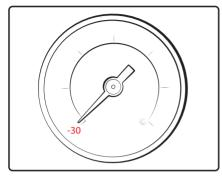
Wait whilst the pressure drops inside the vacuum chamber. The powerful *EC20* will take around 1 minute to reach the high levels of vacuum where degassing starts to occur.
