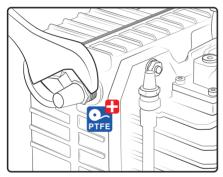
Using a spanner, screw the exhaust silencer into the outlet on the *EC20* vacuum pump.
