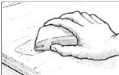
Figure 23 Sand cured fairing compound to desired contour.
